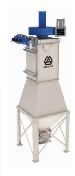
Dust collector P1500/9/R is a box-shaped device. It is used for local filtration - dedusting of storage silos, belt conveyor transfer points, welding operations etc. It is equipped with the support legs, dust hopper and rotary valve.
