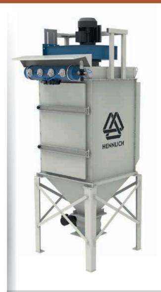
Dust collector P1200/16/R is a box-shaped device. It is used for local filtration - dedusting of storage silos, belt conveyor transfer points, welding operations etc. It is equipped with the support legs, dust hopper and rotary valve.
