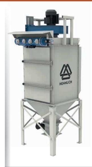
Dust collector P1200/25/R is a box-shaped device. It is used for local filtration - dedusting of storage silos, belt conveyor transfer points, welding operations etc. It is equipped with the support legs, dust hopper and rotary valve.
